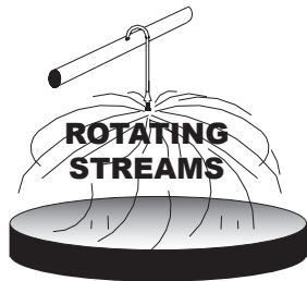
Even distribution throughout full coverage area produces low instantaneous application rates.
