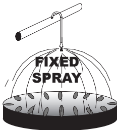
Fixed streams produce high instantaneous application rates on a small percent of area.
